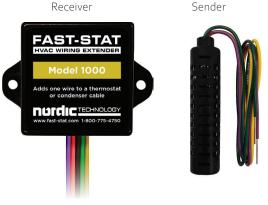
The Sender is installed at the thermostat. The Receiver is installed at the HVAC equipment. They are connected together through the thermostat cable.
